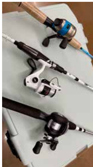
The three basic reels are (from top to bottom) spincast, spinning and baitcast.
