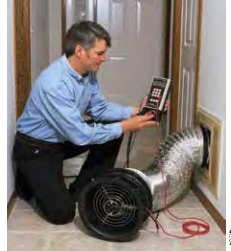
HVAC technicians or energy auditors can use diagnostic equipment to measure air leakage and air flow.
